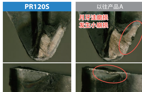
切削参数: V_c = 150 \text{ m/min} , a_p = 1.0 \text{ mm} , f = 0.08 \text{ mm/rev} , Wet SUS316L DCGT11T304型
